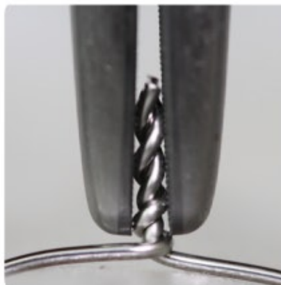
Manual twisting weakens the wire at the base of the twist, where it is most likely to break
